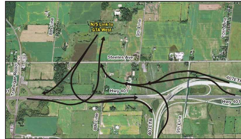
Conceptual GTA West transportation corridor and Highway 401 / 407ETR Interchange (only Freeway to Freeway ramps are shown)
